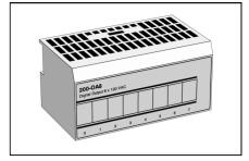
I/O unit for eight digital 120 V AC output signals. The status of each output signal is indicated by a yellow LED.
