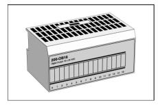
I/O units for 16 digital output signals. The outputs of 200-OB16P are shortcircuit proof. Up to four outputs can be connected in parallel (the total load must, however, not exceed 1.8 A).
