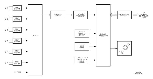
Figure 11-8—RTD Input Module Block Diagram
