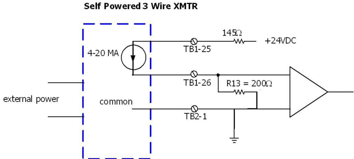
**Note:** TB1: This is done through a 145 ohm resistor inline with a Positive Temperature Coefficient (PTC) device that acts like a fuse (but never needs replacement). Thus, these field terminals can be permanently
