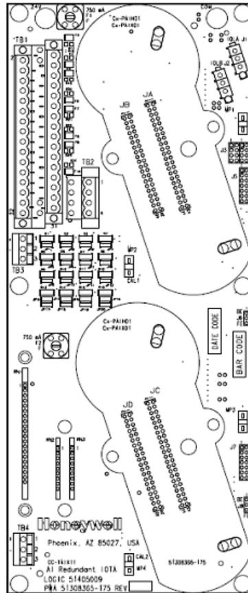
Figure 14: Series C Analog Input 12 inch, redundant IOTA
