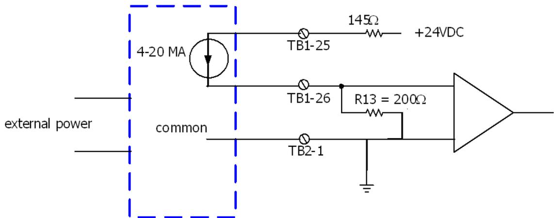
**Note:** TB1: This is done through a 145 ohm resistor inline with a Positive Temperature Coefficient (PTC) device that acts like a fuse (but never needs replacement). Thus, these field terminals can be permanently shorted to ground without damage. This is an improvement over Process Manager due to the inclusion of the PTC device.
