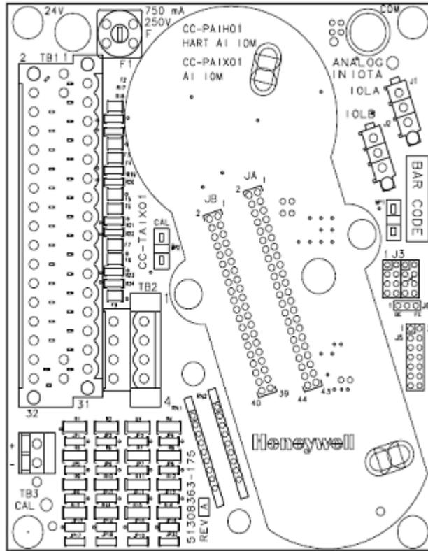
Figure 12: Series C Analog Input 6 inch, non-redundant IOTA
