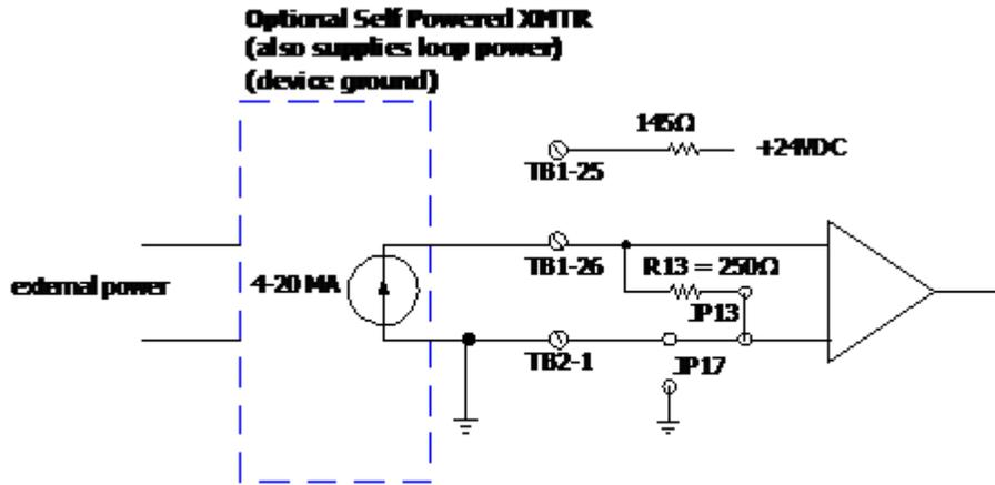
*Self-powered 3-wire transmitter (system ground)*
